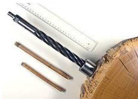
Fig. 12.2.10 Drill for dendrochronology sampling and growth ring counting
