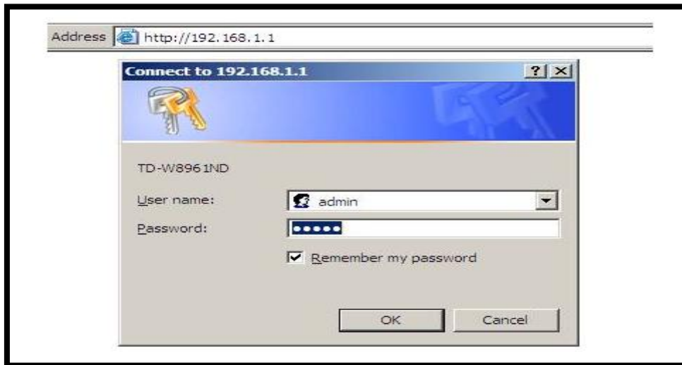
Figure 20: Configuring wireless router
