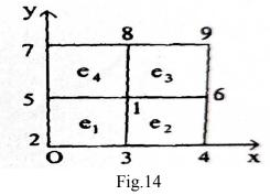
In Fig.14, the mesh shows four rectangular elements contributing at 1. Boundary values remain consistent, with an additional value  $U_4 =$  $U(1,0) = \frac{1}{12} = U_7$ . The apex node is labeled as *i*, while the remaining nodes j, k and m are numbered counterclockwise. Shape functions The shape functions  $N_i$ ,  $N_j$ ,  $N_k$  and  $N_n$  are written as(from equation 14)
