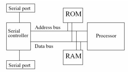
Figure 8.4: Embedded system example.
