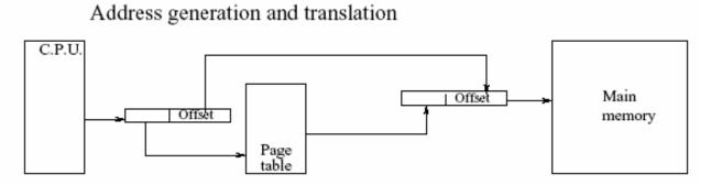
The Offset is same because the page and frame size are same The page table provides the mapping of virutal page to frame number
