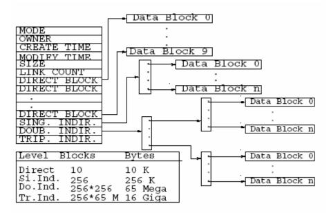
Figure 2.6: Storage allocation in Unix.
