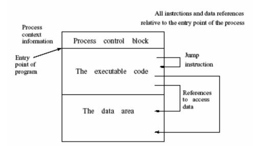
**Figure 4.1: The relocation concept.**
