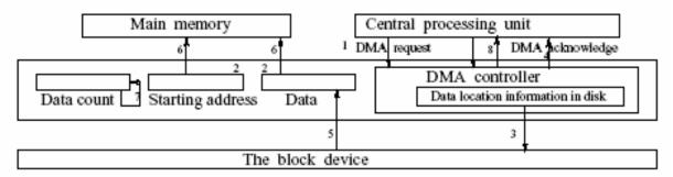
The DMA controller has request, acknowledge, interrupt and read / write lines of control
