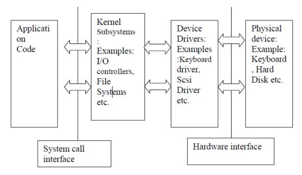
Almost every system call eventually maps to a physical device. With the exception of the processor, memory and a few other entities, all device control operations are performed by code that is specific to the device. This code as we know is called the device driver.
