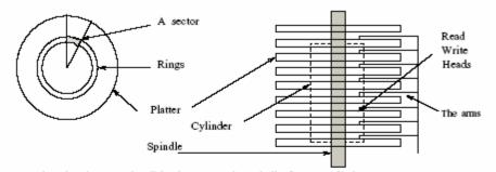
Note that the rings on the disk platters on the spindle form a cylinder. Since all heads are on a particular ring at the same time, so it is easy to organise information on a cylinder. The information is stored in the sectors that can be identified on the rings. sectors are separated from each other. All sectors can hold equal amount of information.
