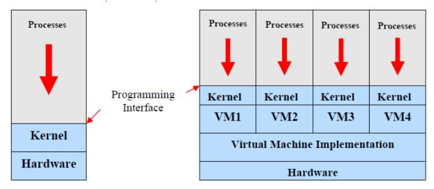
System models. (1) Non-virtual machine. (2) Virtual machine.
