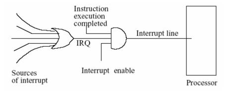
Figure 5.3: How an interrupt is detected.
