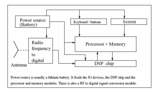
Figure 8.6: A typical hand-held device architecture.
