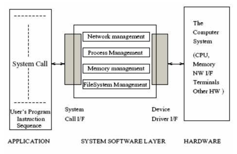
Figure 7.1: Processing system calls.
