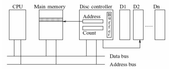
Figure 5.6: DMA : Hardware support.
