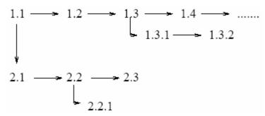
Figure 17.1: A typical version tree under SCCS.
