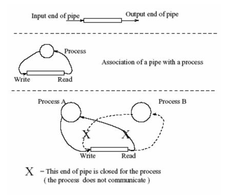
Figure 7.2: Pipe as an IPC Mechanism.
