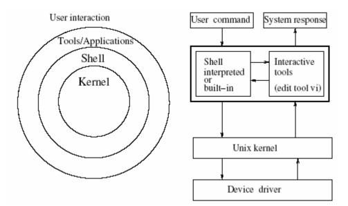
Figure 13.1: A Unix system shell.
