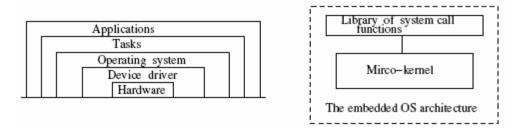
Figure 8.5: Software view of microkernel based OS.
