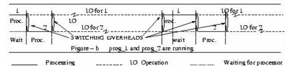
In the light of the above let us briefly review this figure above. In a uni-programming system (figure a) we have one program engaging the processor. In such a situation the processor is idling for very long periods of time. This is so because IO and communication to devices (including
