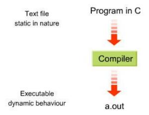
In other words, To begin with let us define what is a "process" and in which way a process differs from a program. A process is an executable entity – it's a program in execution. When we compile a C language program we get an a.out file which is an executable file. When we seek to run this file – we see the program in execution. Every process has its instruction sequence. Clearly, therefore, at any point in time there is a current instruction in execution.
