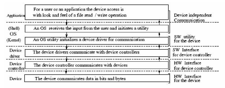
Figure 5.8: Communication with IO devices.
