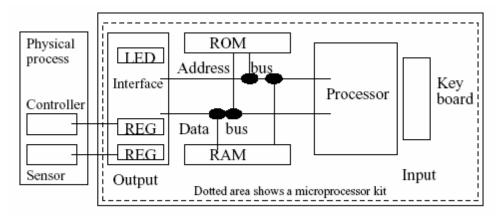
Figure 8.3: Embedded system architecture.
