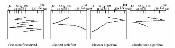
In FCFS policy the information seek takes place in the sequence of cylinder numbers which are in the request queue. In figure 5.15 we plot map for FCFS access. In all the examples we assume that the arm is located at the cylinder number 100. The arm seek fluctuates sometimes very wildly. For instance, in our example there are wild swings from 12 to 194 and 41 to 172.
