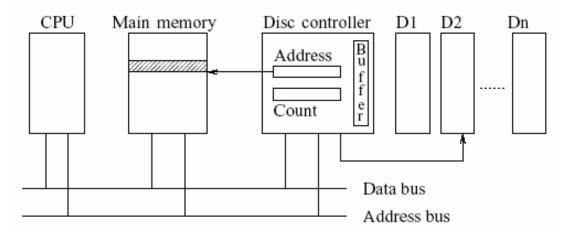
Figure 5.6: DMA : Hardware support.
