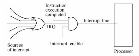
Figure 5.3: How an interrupt is detected.
