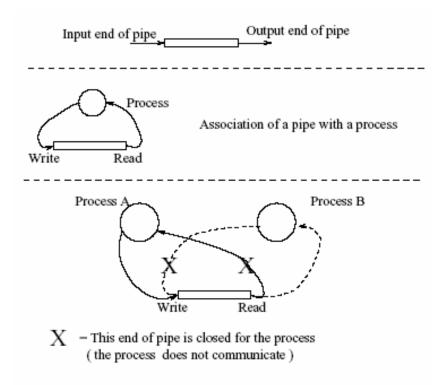
Figure 7.2: Pipe as an IPC Mechanism.
