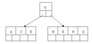
Inserting M requires a split. Note that M happens to be the median key and so is moved up into the parent node.
