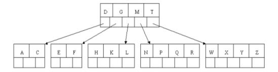
Finally, when S is added, the node with N, P, Q, and R splits, sending the median Q up to the parent. However, the parent node is full, so it splits,
