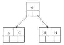
Inserting E, K, and Q proceeds without requiring any splits:
