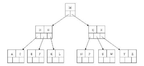
Finally, let's delete E. This one causes lots of problems. Although E is in a leaf, the leaf has no extra keys, nor do the siblings to the immediate right or left. In such a case the leaf has to be combined with one of these two siblings. This includes moving down the parent's key that was between those of these two leaves. In our example, let's combine the leaf containing F with the leaf containing A C. We also move down the D.
