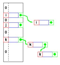
It is the combination of standard and general coalesced hashing. Under this method, the colliding item is inserted to the list immediately following the hash position unless the list forming from that position containing a cellar element.
