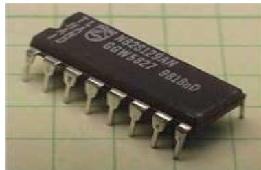
Figure 3.4: Programmable Read-Only Memory (PROM)
