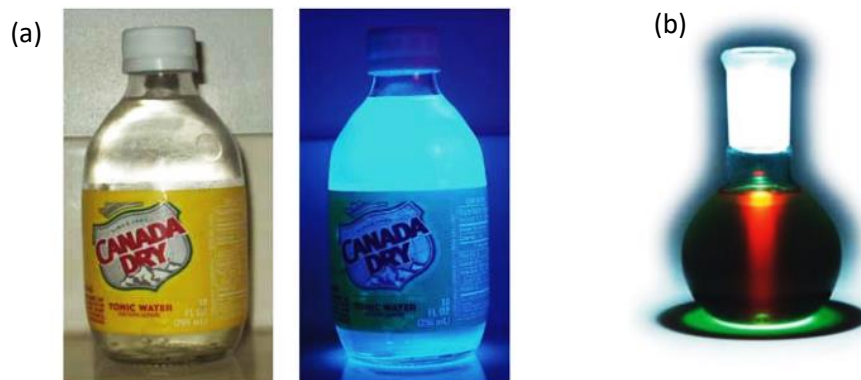
Figure 2.4: (a) tonic water is clear under normal light, but vividly fluorescent under ultraviolet light, due to the presence of the quinine used as flavouring; (b) A solution of chlorophyll in ether solution shown blood red fluorescence.
