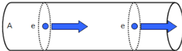
Figure 9.13: Flow of charge carriers
