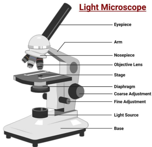
Figure 9.6: Schematic of light microscope.
