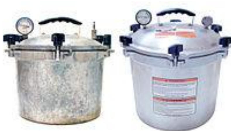
Fig 4.5 Stovetop autoclaves—the simplest of autoclaves
