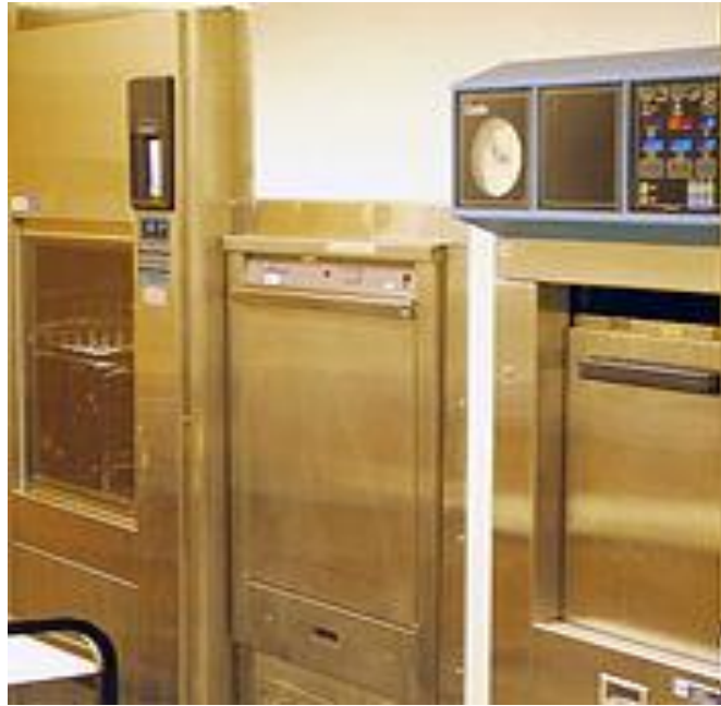
Fig 4.6 The machine on the right is an autoclave used for processing substantial quantities of laboratory equipment prior to reuse, and infectious material prior to disposal. (The machines on the left and in the middle are washing machines.)
