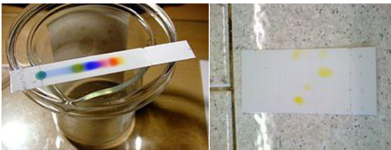
Fig.4.22 Separation of black ink on a TLC plate
