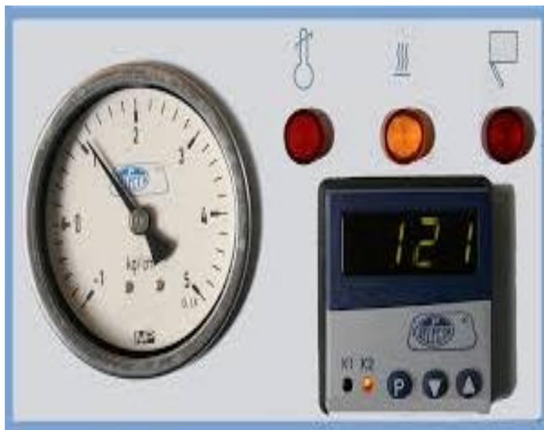
Fig 4.7 The Autoclave must reach 121 degrees Celsius
